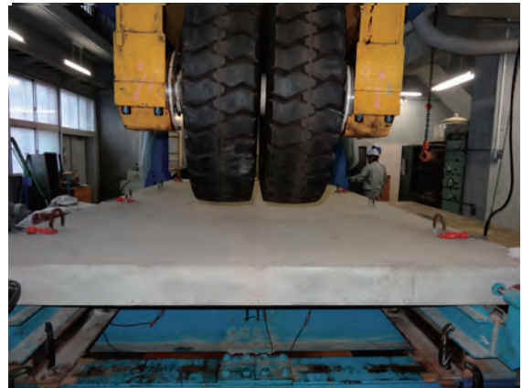
Running wheel loading machine and deteriorated concrete slab
