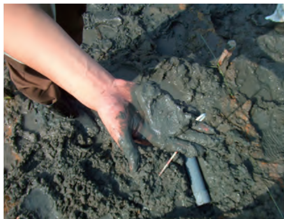
Deteriorated lime-treated clay in a marine environment
