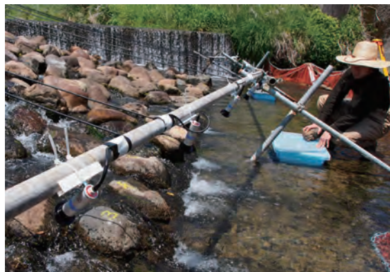
Field experiment in a stone embedded fish way to reveal the relationship between fish migration paths and their physical condition.
